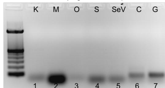
RT-PCR analysis showing silencing of the transgenes KLF4, c-MYC, OCT4 and Sox2 and the absence of Sendai virus in the 5PNF\_TDiPSsv\_PM\_6 iPS line.
